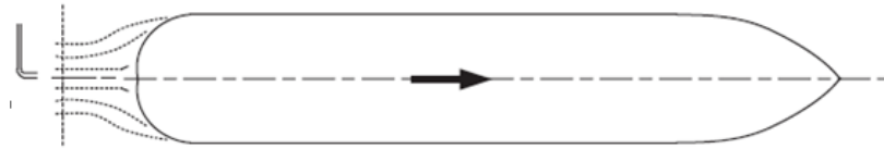
Figure 2-3 Measurement of total viscous resistance [1]
