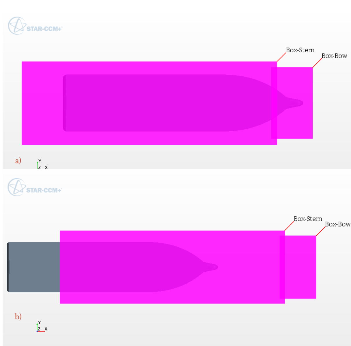
Figure 5-1 Positions of volume controls. a) Scaled model & domain, b) Scaled model & domain (2)
