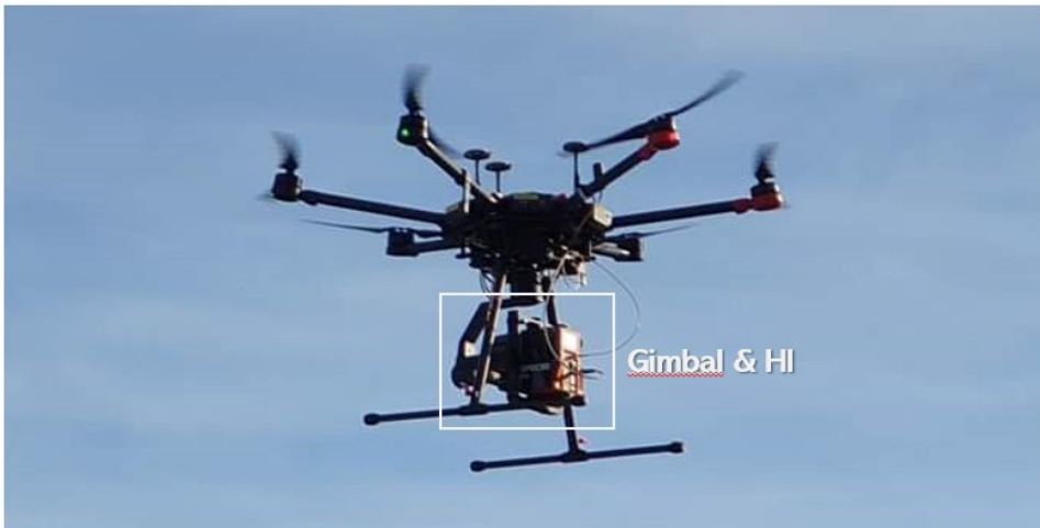
Figure 2.4: The unmanned aerial vehicle (UAV, DJI S1000+) octocopter taking off, carrying the hyperspectral imager (HI, SPECIM AFX10) connected by a stabilizing gimbal (Gremisy T7), at Hopavågen. Photo by Pål Kvaløy.
