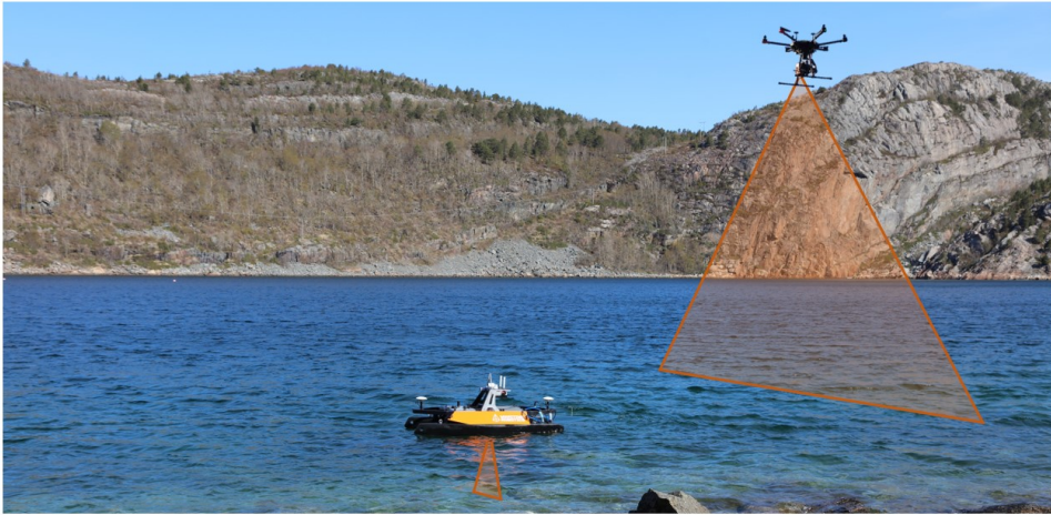
Figure 2.5: An illustration showing the simultaneous hyperspectral mapping surveys performed in Hopavågen, Trøndelag. A USV travels as it images a seagrass meadow. The USV carrying a UHI survey was synchronized with the UAV carrying a HI transect above the seagrass meadow, and the two transects are compared in the results. Photomontage, photos by Pål Kvaløy and Asgeir Sørensen.
