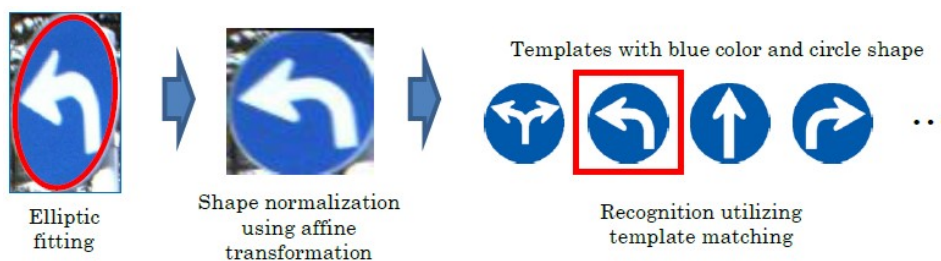
Figure 8: Classification with template matching after shape normalization (Li et al. 2016)
