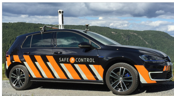
Figure 4.1: The MMS vehicle used to record data (Triona, 2022)
