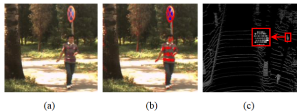
Figure 4: An example of a situation where the laser reflectivity is not very discriminative, but colour is an effective tool to detect traffic signs. (Zhou and Deng 2014)
