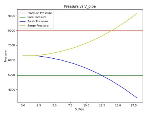
Figure 3-1. Python Output - Pressure versus Tripping Speed
