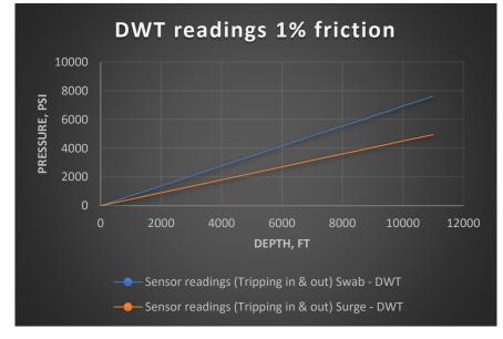
Figure 4-7. DWT sensor readings (1% friction)
