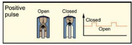
Figure 6-1. Representation of a positive mud-pulse system (Cooper & Santos, 2015)
