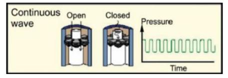
Figure 6-2. Representation of Continuous mud-pulse system (Cooper & Santos, 2015)
