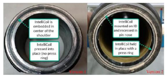
Figure 7-2. Left: Intellicoil's first generation. Right: Intellicoil's second-generation (Sehsah et al., 2017)
