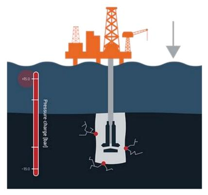
Figure 5-3. Heaving Downwards. (Kvernland, 2019)
