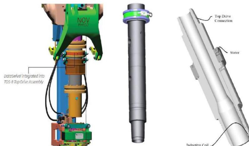
Figure 2-3. Data swivel; Intelli Coils. (Babu, 2019)
