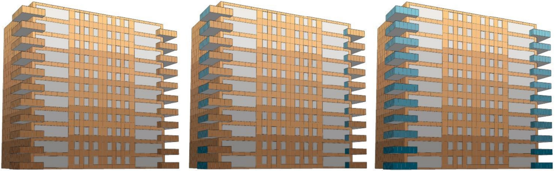
Figure 38. FIPV design for high-rise with side large balconies, in main yellowish hue Y30R and the corresponding complementary hue
