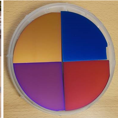
Figure 2.25: Coloured prototypes with thin-films applied on top of flat Si wafer solar cells, from Ørnulf Nordseth. 21
