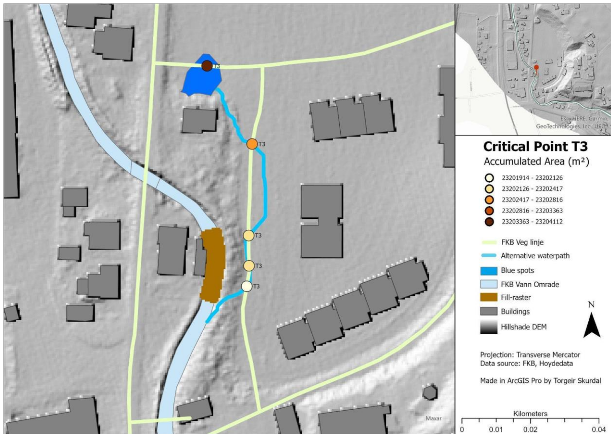
Figure 6.22: Showing the indicated damage caused to roads by critical point 3, from running the model.
