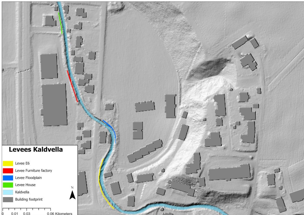
Figure 6.11: Showing levees that have been added, based on collected GPS points.
