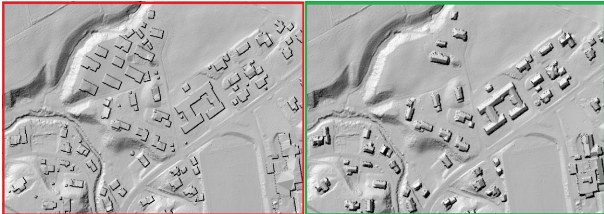
Figure 6.4: Comparing buildings included in the FKB building data from 2021 (left) and LiDAR data from 2015 (right).
