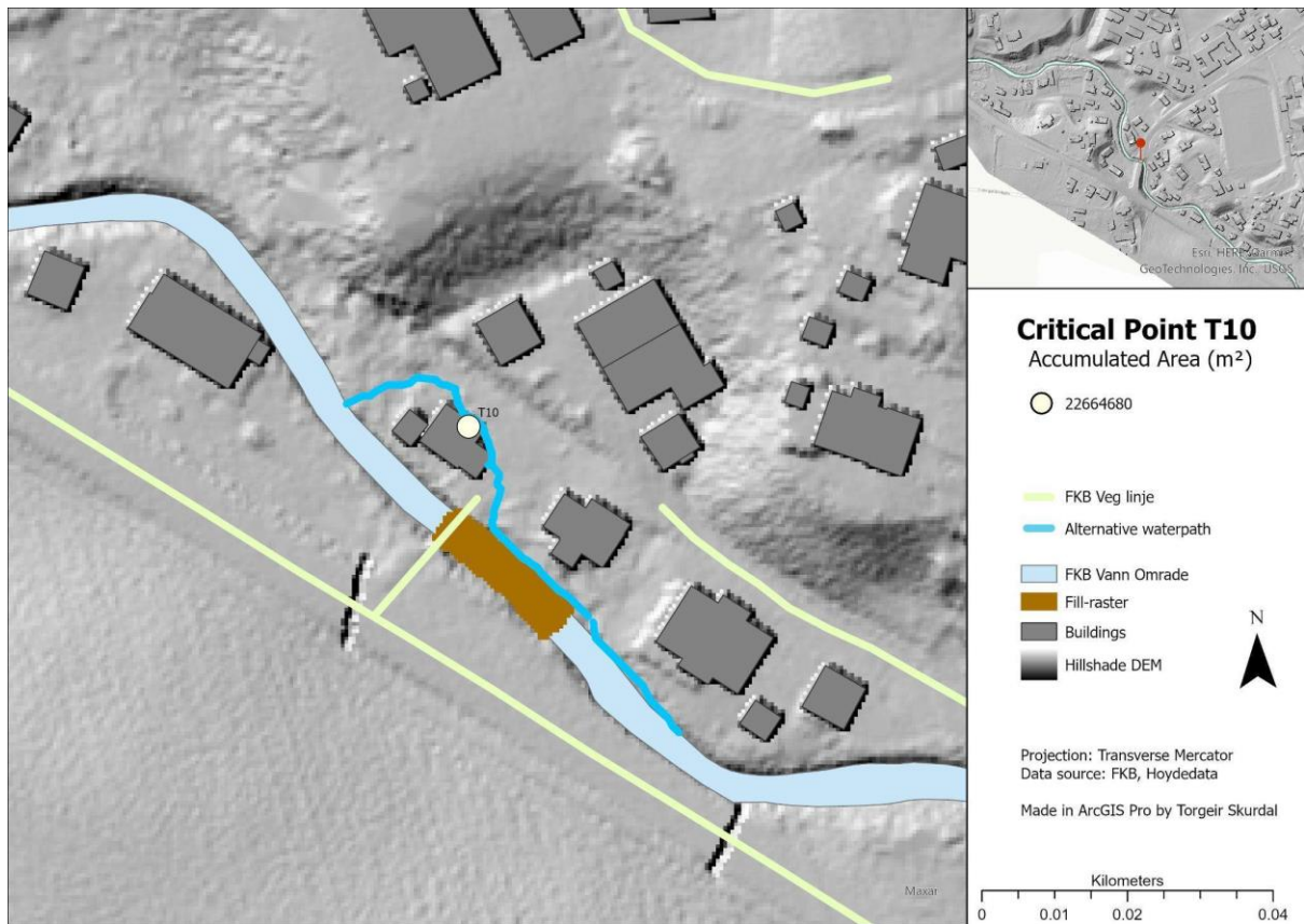
Figure 6.46: Showing the indicated damage caused to buildings by critical point 10, from running the model.
