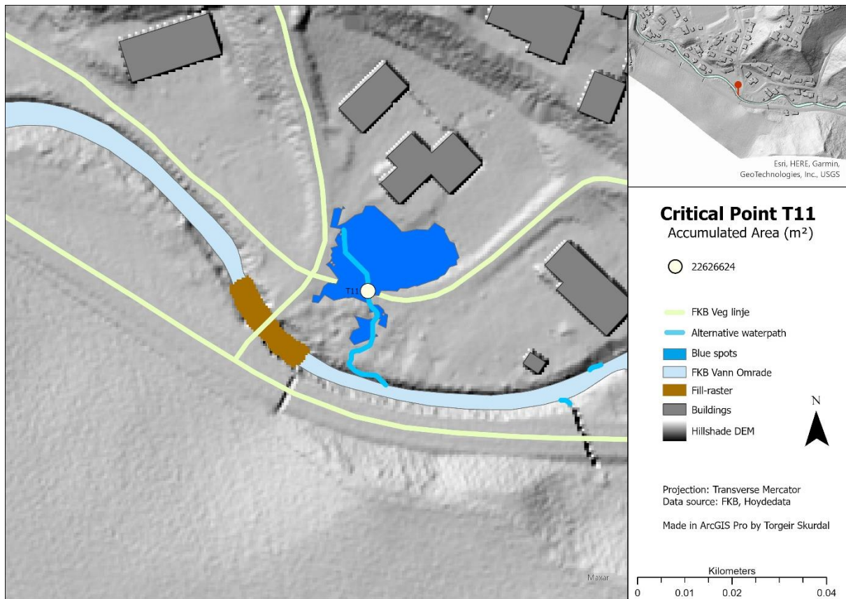
Figure 6.49: Showing the indicated damage caused to roads by critical point 11, from running the model.
