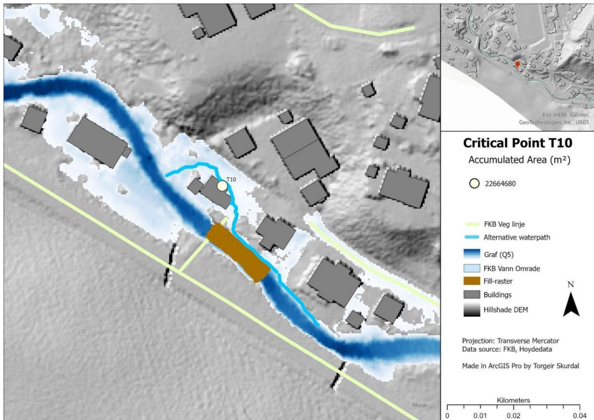
Figure 6.48: Showing the modeled damage caused to buildings by critical point 10, compared to Flood map by Graf (2021).
