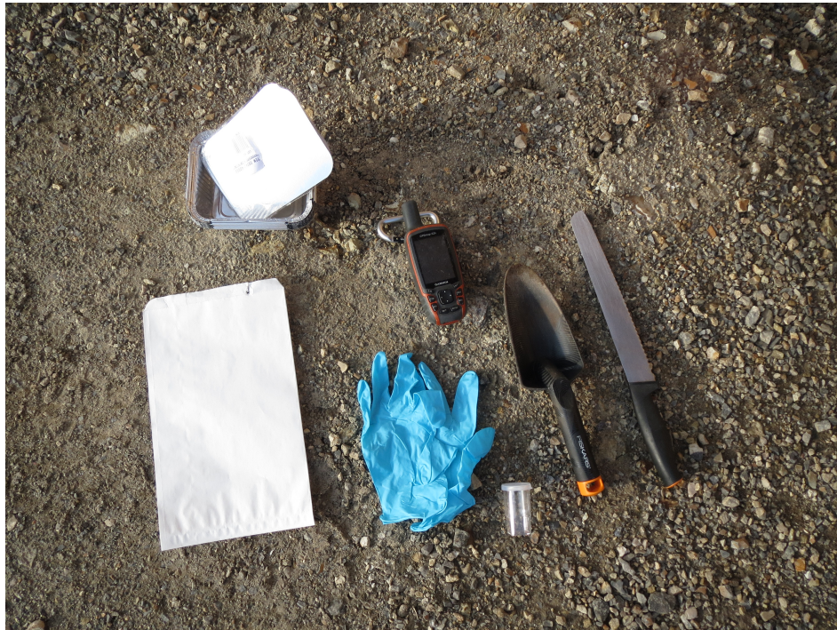
Figure 10: The sampling equipment used for soil and guano samples. From right to left: paper bags, aluminium boxes, nitrile gloves, GPS, CC-cups, garden trowel and common bread knife in stainless steel. Credit: Mathilde K. Syvertsen
