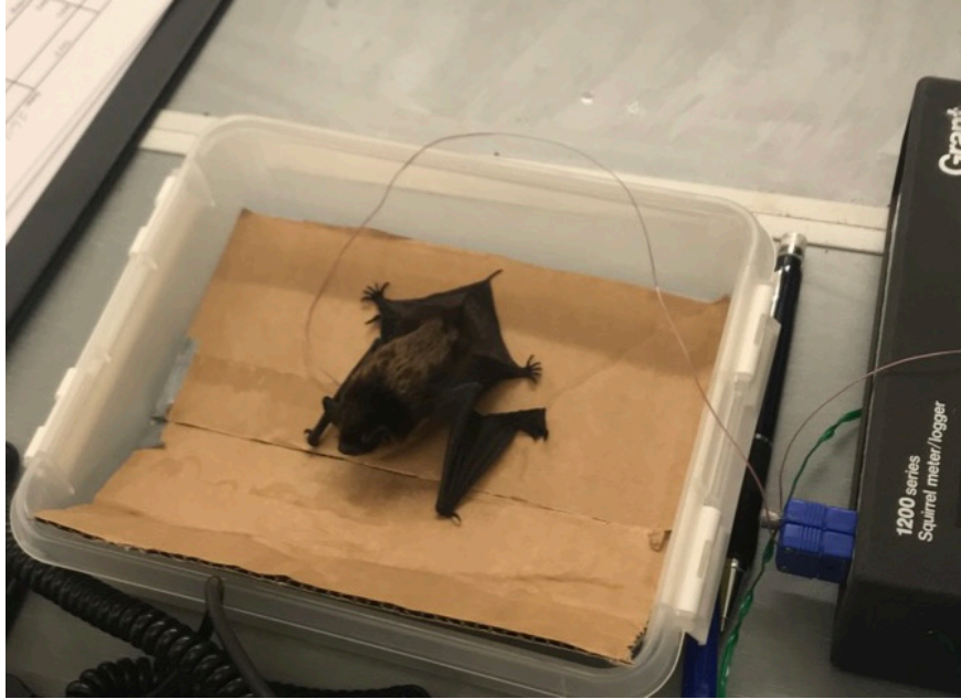
Figure 2.1: The laboratory setup used in the study. E. nilssonii was placed with ventral side down on a cardboard plate inside a plastic box, with the wire of the thermocouple (1200 series Remote Squirrel Meter/Logger, Grant Instruments Ltd., Cambridge, UK) taped to its abdomen.
