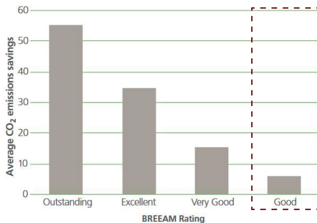
Figure 32: Avg CO2 emissions savings associated with different BREEAM Ratings (Taylor, no date)
