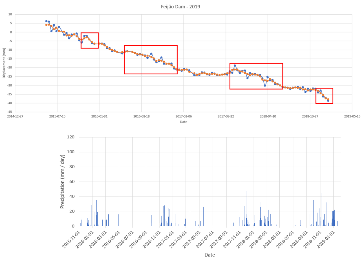
Figure 22: Surface displacement over time and precipitation data over time in the Córrego do Feijão tailings dam (NGI; Visual Crossin Weather, 2021).
