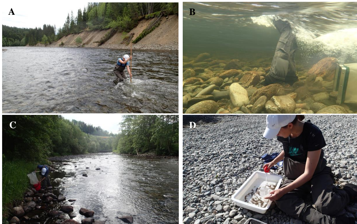
Figure 2. Resampling of the rivers Verdalselva (A, B), Homla (C), and Skauga (D). During a transect (A), the upper layer of the river sediments is disturbed by kicking, and loosened benthic invertebrates are caught by the net (B). The contents in the net are place transferred to a bucket (C), and living organisms are sorted out and placed in a container with ethanol (D). Photo: Gaute Kjørstad.
