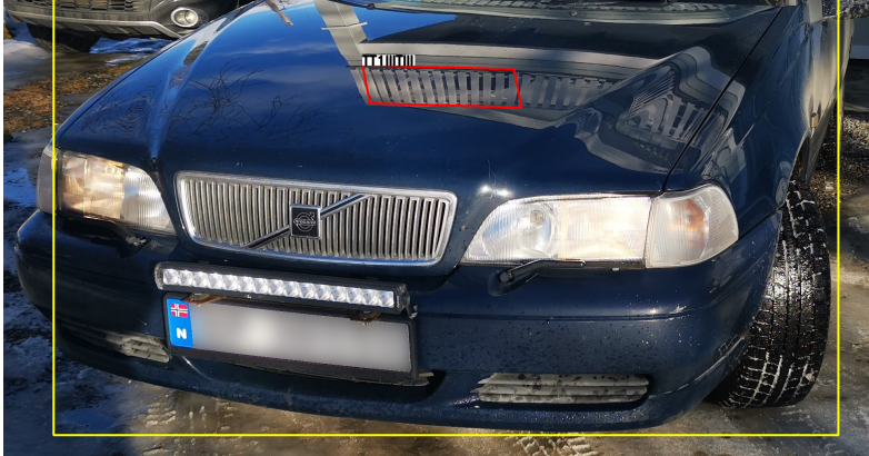
Figure 5.14: Reflection detected as license plate..
