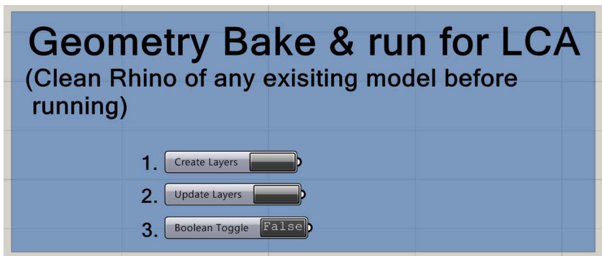
Figure 3.13 Bombyx tool panel for the user. The sequence is essential to get accurate data
