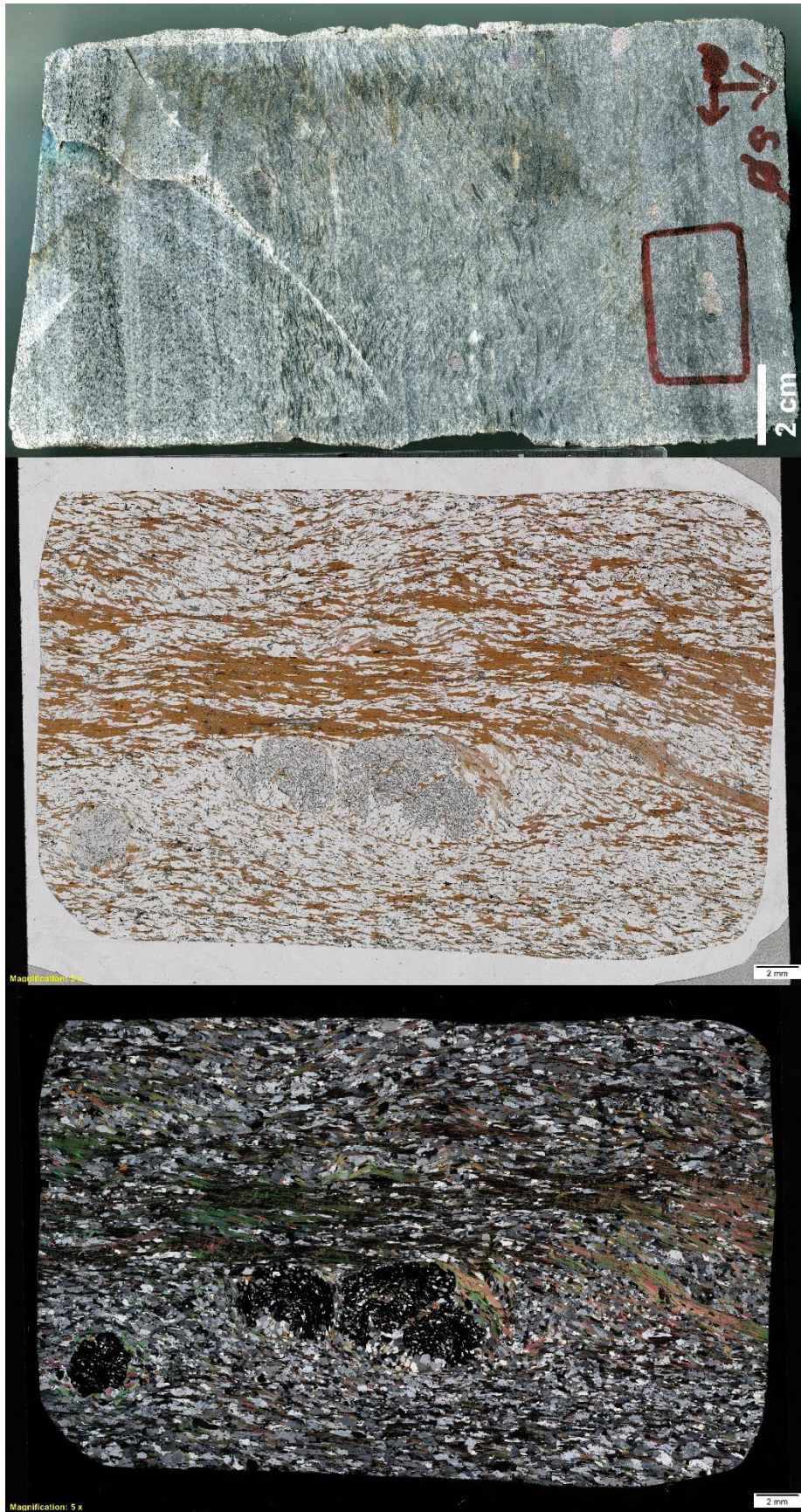
Rock slab, and thin section scans of gmf2020-30. PPL in the middle, XPL, bottom.
