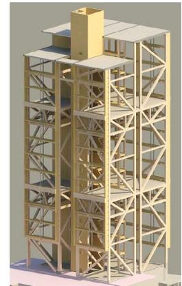
Figure 8 Structure of Treet with Trusses columns (Kato,2014)
