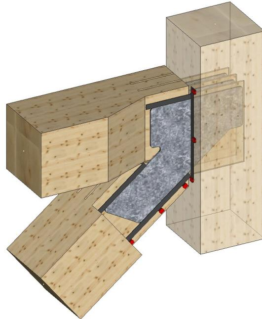
*Figure 25 Steel plates incorporated into Glulam Structure (Rune Abrahamsen,2017)*
