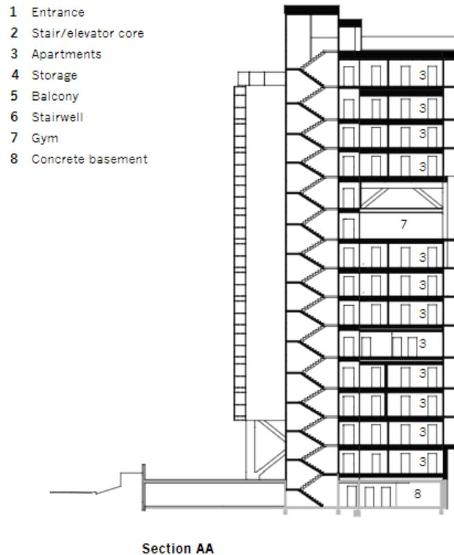
The bedrock is about 5 m below the basement floor. Over 100 vertical and slanted steel core piles are driven into the bedrock to serve as the building's foundation. Some of the piles will have to withstand tension strains as well. When the building is subjected to wind loading, tensile forces can be applied to some of the diagonals and columns. These forces are conveyed to the ground by using slotted-in steel plates and dowels to connect the glulam columns to the concrete foundation.
