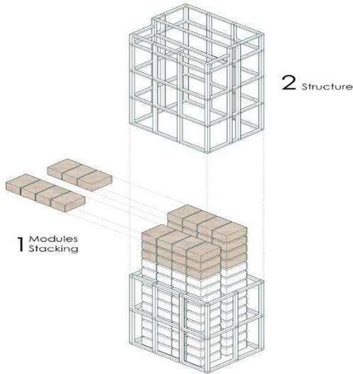
Figure 7 : Volumetric Hybrid systems
