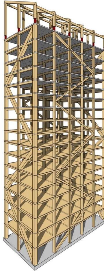
Figure 23 Structural system of Mjøstårnet
