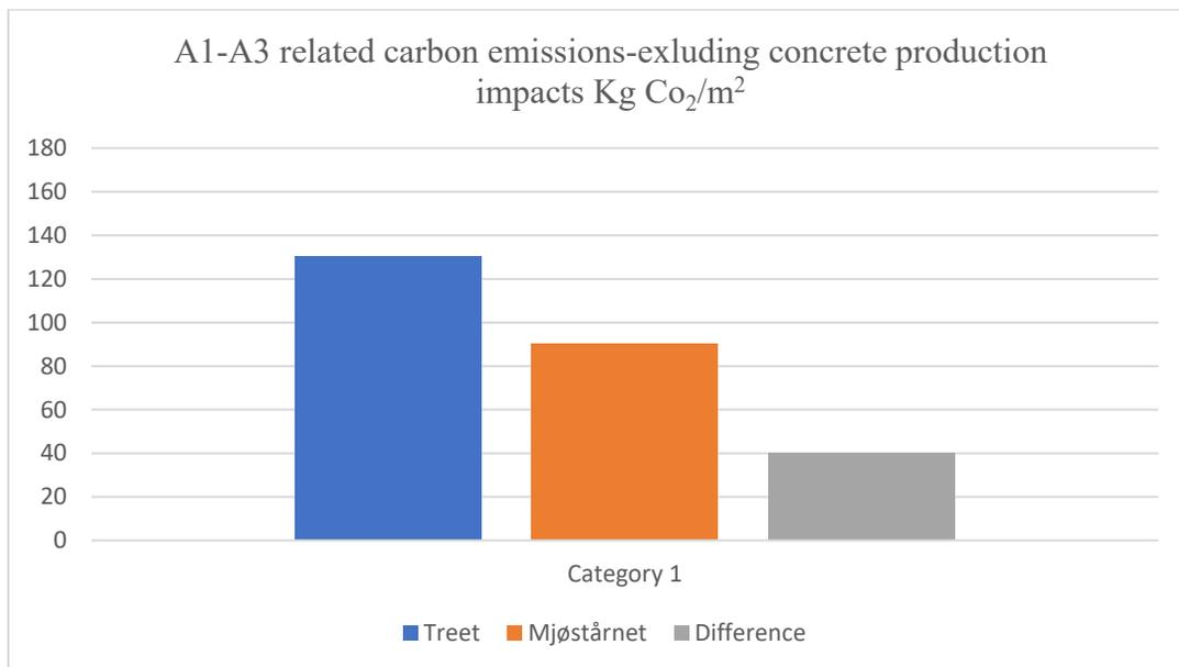
This Figure shows GHG emissions for module A1-3 of the reference buildings, the results show that if we exclude the concrete from the evaluation, the Treet would be responsible for more GHG with a value of 760615.6 Kg Co<sub>2</sub>, which is 25 % higher than Mjøstårnet when in the production phase. While Mjøstårnet carbon emissions drop by half when excluding concrete masses.
