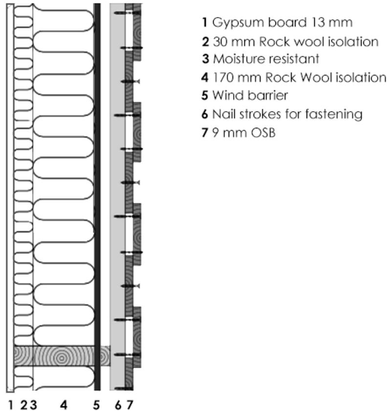
Figure 27 Example of a detail section of a Prefabricated sandwich timber panel.
