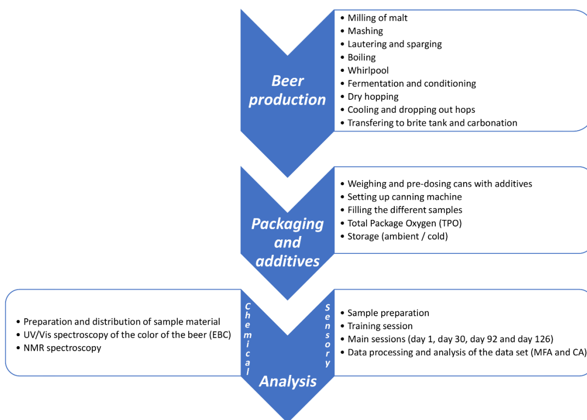
Figure 3 - Flow chart of the experiment presented as the sequence of steps
