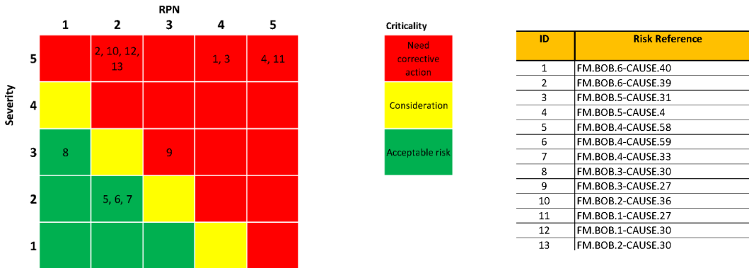
Fig. 4. Risk matrix for BOB failure modes. The RPN is referenced to a scale of 100, and then into ranges of 20 to give the resulting 1-5 indexing .
