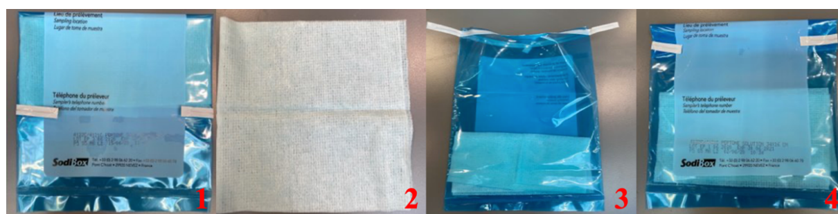
Figure 7 – Sample cloth used in study. 1, unused cloth in bag. 2, the sterile sample cloth. 3, sample cloth put back in bag after sampling. 4, bag with used sample cloth is sealed by folding the bag three times and fastening the white strips.
