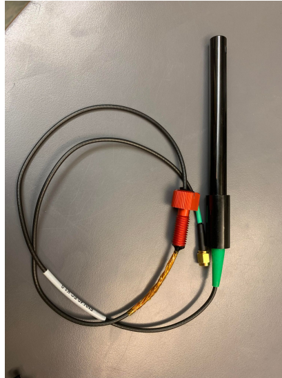
Figure 5.7: The result from rehousing and potting on the conductivity sensor
