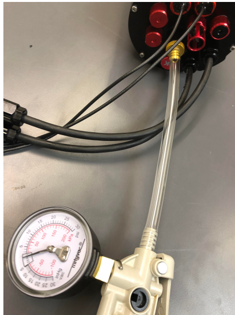
Figure 3.5: The hand pump connected to the valve on the lid
