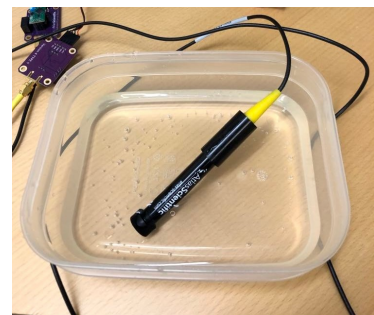
Figure 3.2: Functionality test dissolved oxygen
