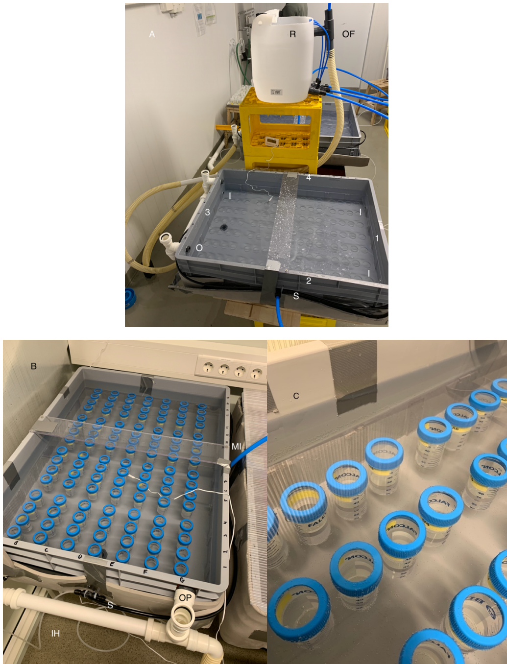
Figure 4. Incubator set up. A: Intake water was transported to the reservoir (R) fitted with an overflow (OF). Blue hoses were the main inlet hoses transporting water from the reservoir to the incubator. Inlet water was first split in two directions to sides 1 and 3 via the splitter (S) before reaching another splitter which divided the water to the inlet hoses as shown in B) and into the incubator through the bottom. Outflowing water went through the outflow (O). B: Overview showing the main inlet (MI), how the water was split in two (S) and the inlet hose (IH) transporting the water into the incubator. Outflowing water went through the outlet pipe (OP). C: Close-up of incubator tubes fitted with mesh in top and bottom. Photos: Anna S. Båtnes and Mikael Furberg.
