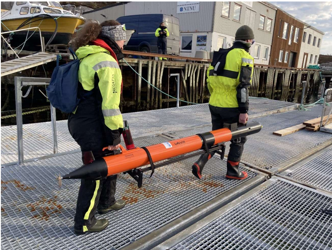
Figure 1: LAUV (Light Autonomous Underwater Vehicle) Roald carried by Maren Thu and Andreas Våge at Mausund Field Station prior to deployment. Photo: Annecken Nøland.
