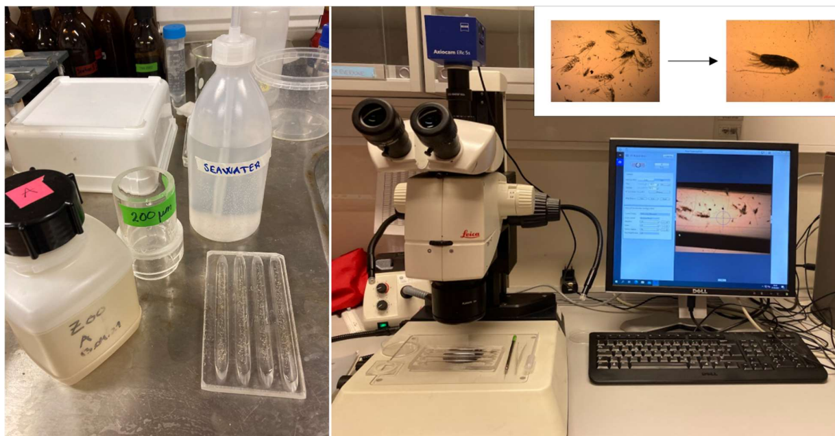
Figure 11: Net sample analysis. Left: Sample M1A and a subsample, including the sieve (200 \mu\text{m} ) and seawater used to obtain it. Photo: Annecken Nøland. Right: The stereomicroscope with camera system (AxioCam ERc 5s) attached at the top, enabling images of separate individuals to be obtained (see inset photo). Photo: Annecken Nøland.
