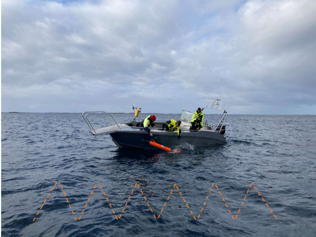
Figure 8: Launching of the LAUV by the AILARON team from motorboat at Mausund, and visualization of the yoyo transect (orange). Photo: Annecken Nøland
