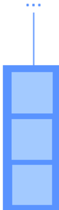
Figure 2.3: Vertical scaling. A single PC is upgraded with more powerful hardware.
