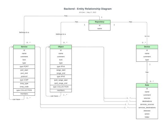
Figure 28: Entity Relationship Diagram. The figure shows the relationships between the models that exist in the REST API
