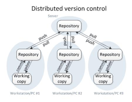
Figure 2: Workflow of a distributed version control system. Developers clone a repository locally, and make commits and updates to their local repository. Changes are later pushed or pulled from the central repository [10]
