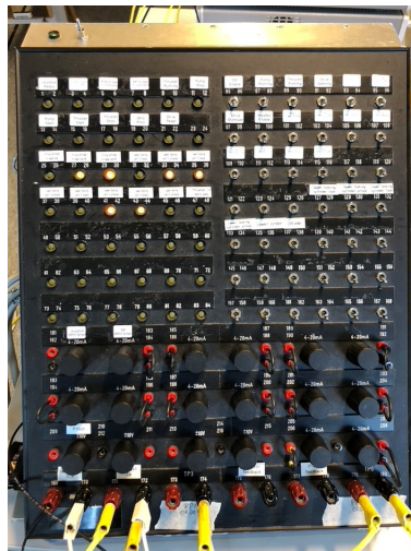
Figure 5.3: Test jig for simulating signals and feedback.
