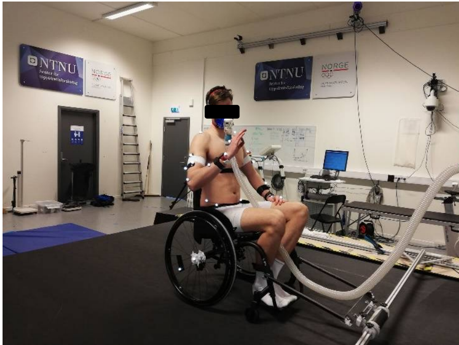
Figure 2. Data collection setup representing the attachment of the wheelchair to the safety bar on rails, and reflective markers. The mouthpiece was used for the cardiorespiratory data collection, which was not used for this project.
