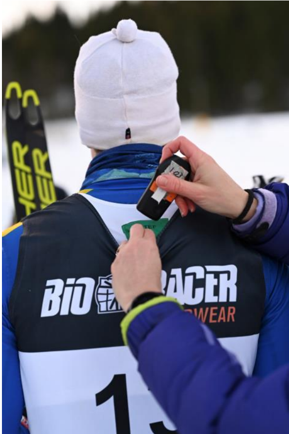
Fig. 5. Sensor placed in a pocket of a customized bib before each race.
