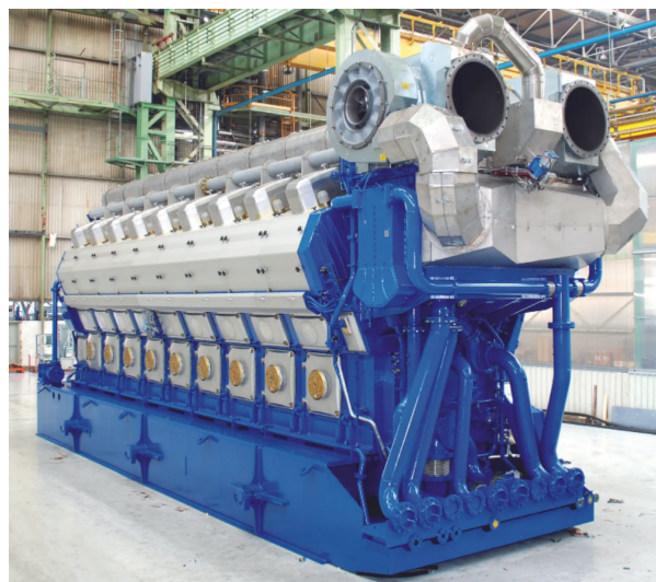
Figure 3.3: A dual-fuel engine designed and produced by Wärtsilä [108]
