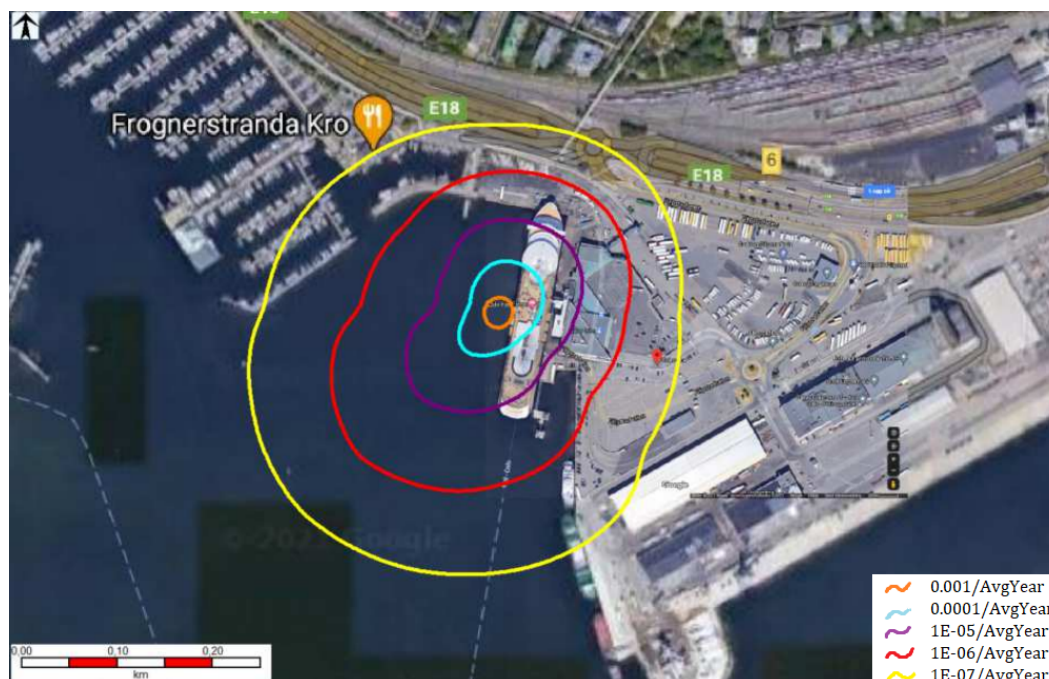
Figure 3.1: Location Specific Iso-Risk contour of an ammonia powered passenger vessel. Modified from [94]
