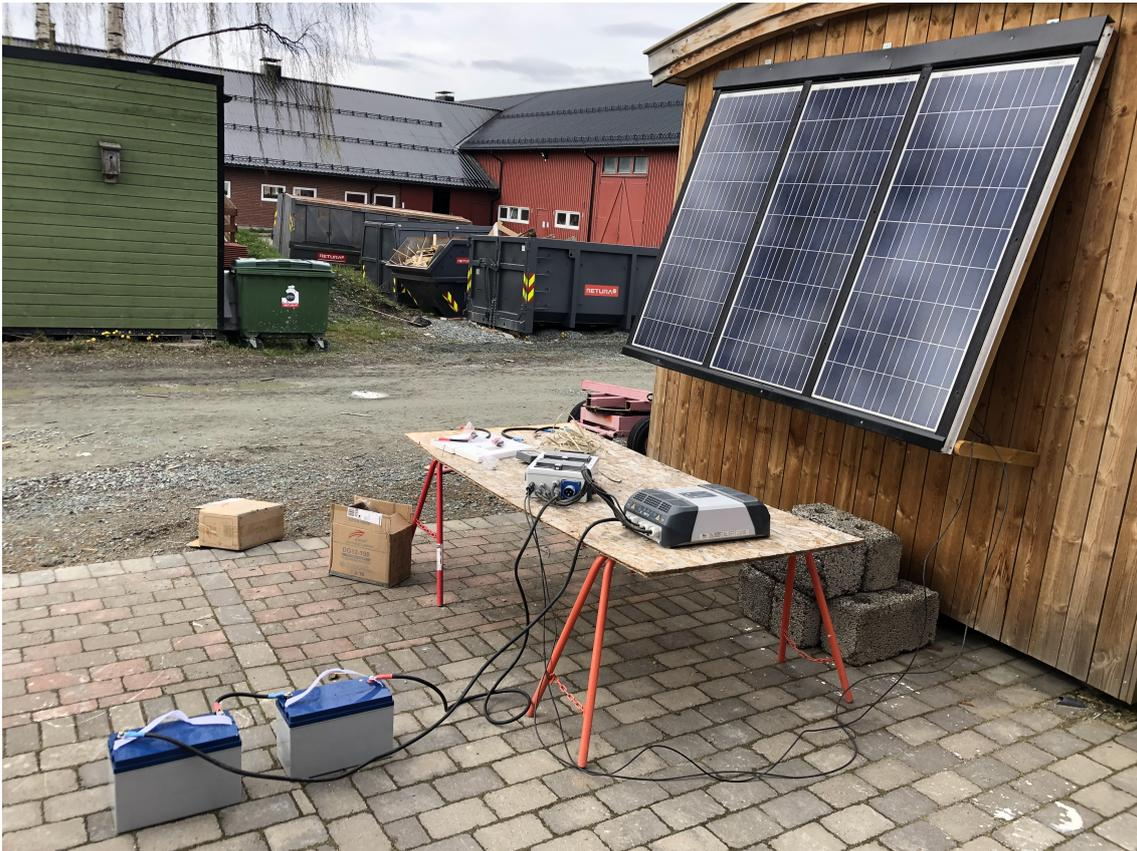
Figure 23: Testing of the MPPT and inverter
