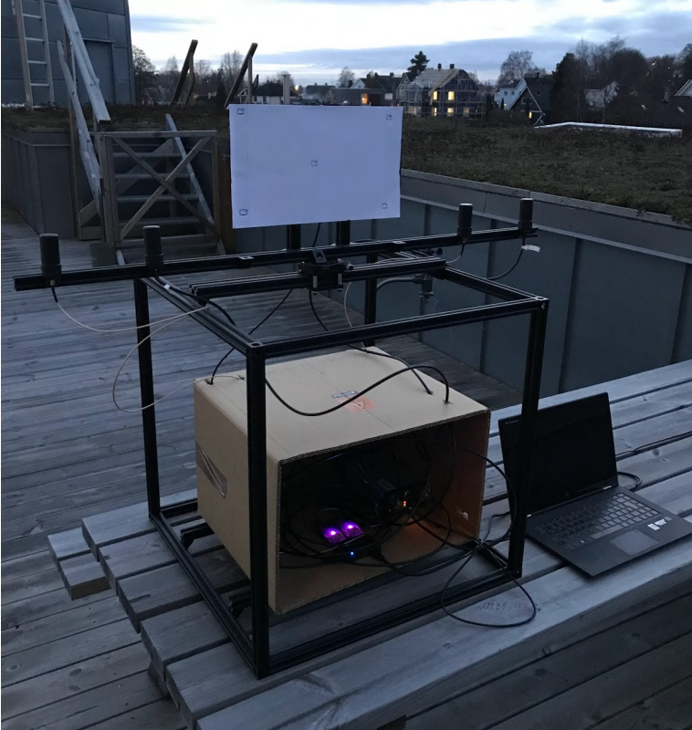
Figure 5.7: Rig setup with mounted circuit board and GNSS antennas.
