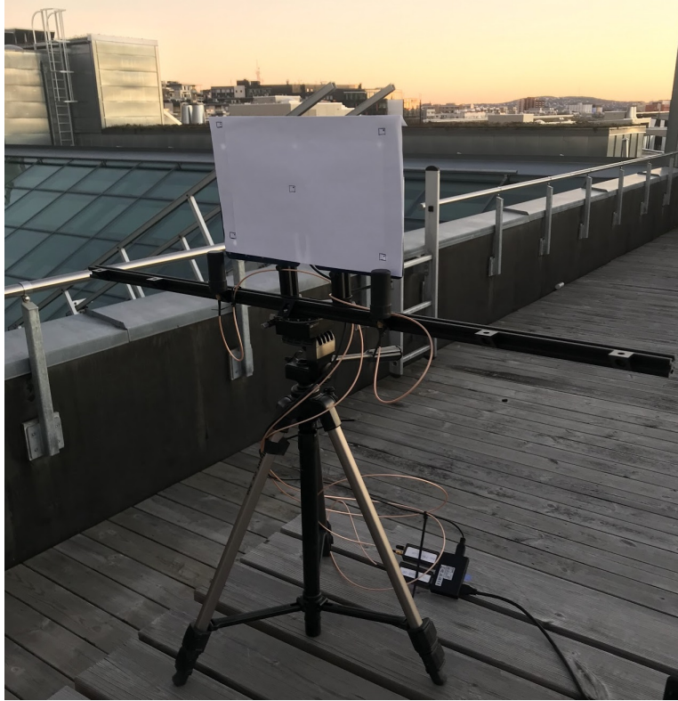
Figure 5.8: Rig setup with mounted circuit board and GNSS antennas for tripod.
