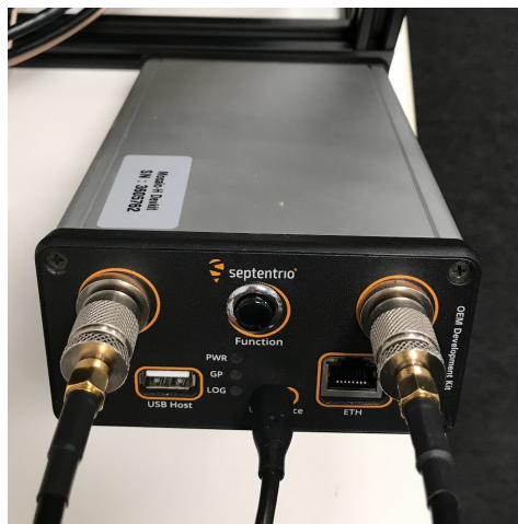
Figure 2.3: Mosaic-H developer kit from Septentrio.
