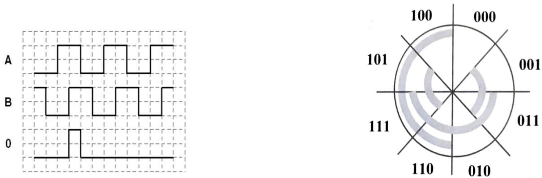
(a) Pulse train using channel A, B and 0 in an incremental encoder
