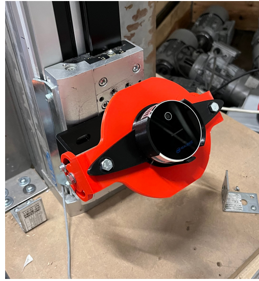
(b) L515 camera mounted on the linear axis, and located in the bottom position.
