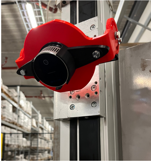
(a) L515 camera mounted on the linear axis, and located in the top position.
