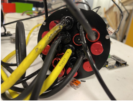
(a) Photo of cable entry points
