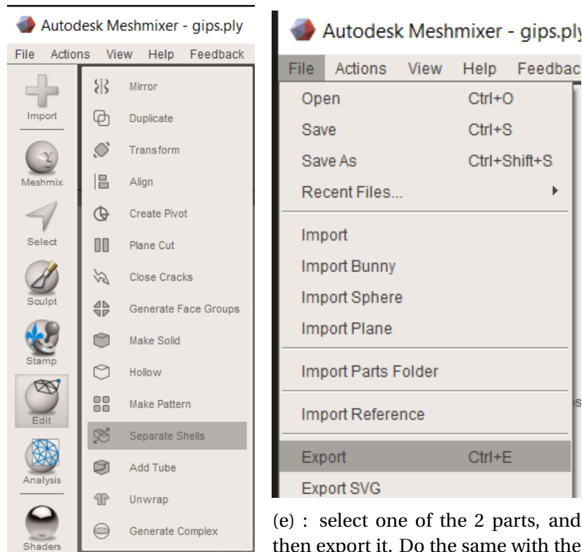
Figure 2: After this is done, convert the 2 parts into .step files, prusaSlicer was used to do this. After that just 3d print the step file
