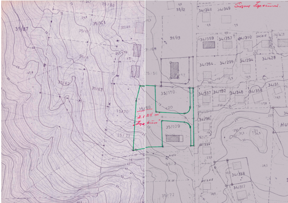
Figure 3.1: Information loss in a digitized map. The left side is a properly scanned version and the right side has a loss of information.
