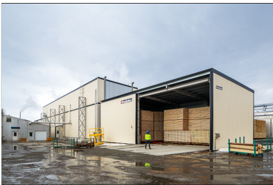
Figure 1: Example image showing the drying kiln used by Moelven in order to dry wood ( Moose River 2019 )
