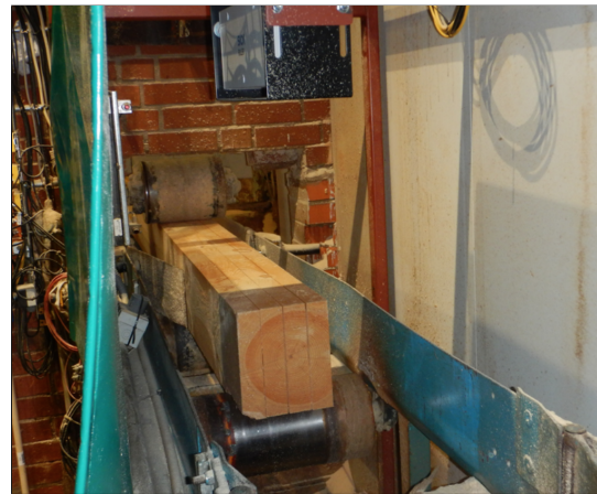
Figure 23: Heartwood cut accordingly to the saw set. Picture taken by project member during visit to the sawmill.
