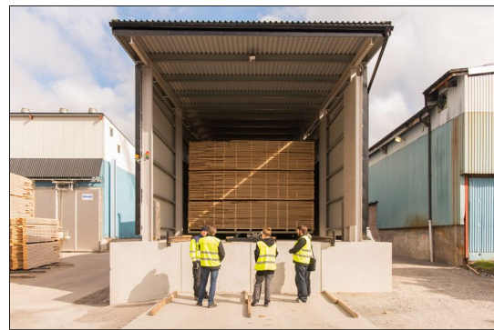
Figure 2: Example image showing the drying kiln used by Moelven in order to dry wood ( FB continuous kiln 2017 )
