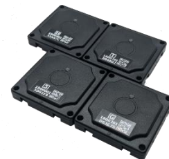
Figur 3 IBS05 Bluetooth low energy Beacon/tag
