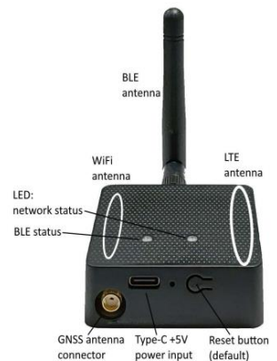
Figur 16 IGS03M Antenne arkitektur, bilde funnet i dokument: https://www.ingics.com/doc/Gateway/GW0038_Beacon_Gateway_i_GS03W_E_M_User_Manual.pdf
