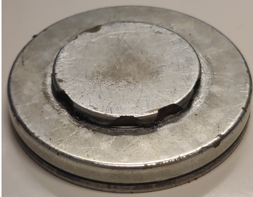
Figure 5.10: Damages on the levitating magnet
