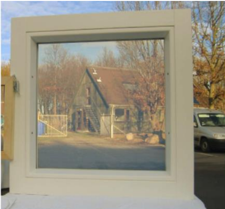
Figure 4.3: Example of an evacuated aerogel glazing consisting of monolithic aerogel. The view through is clear, although some haziness is present. The window is not exposed to direct sunlight (Schultz & Jensen, 2007).
