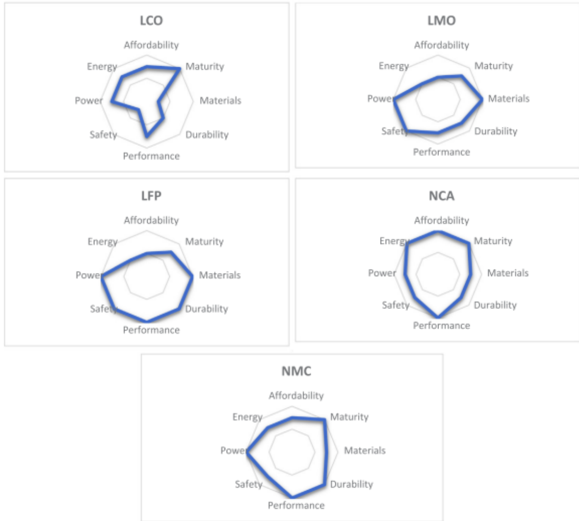
Figure 3: Main characteristics of the most common LIB chemistries. Reprinted from Zubi et al. [20].
