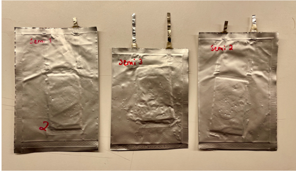
Figure 44: Three semi-solid state cells, the middle one having long enough tabs for formation and HPPC-testing.
