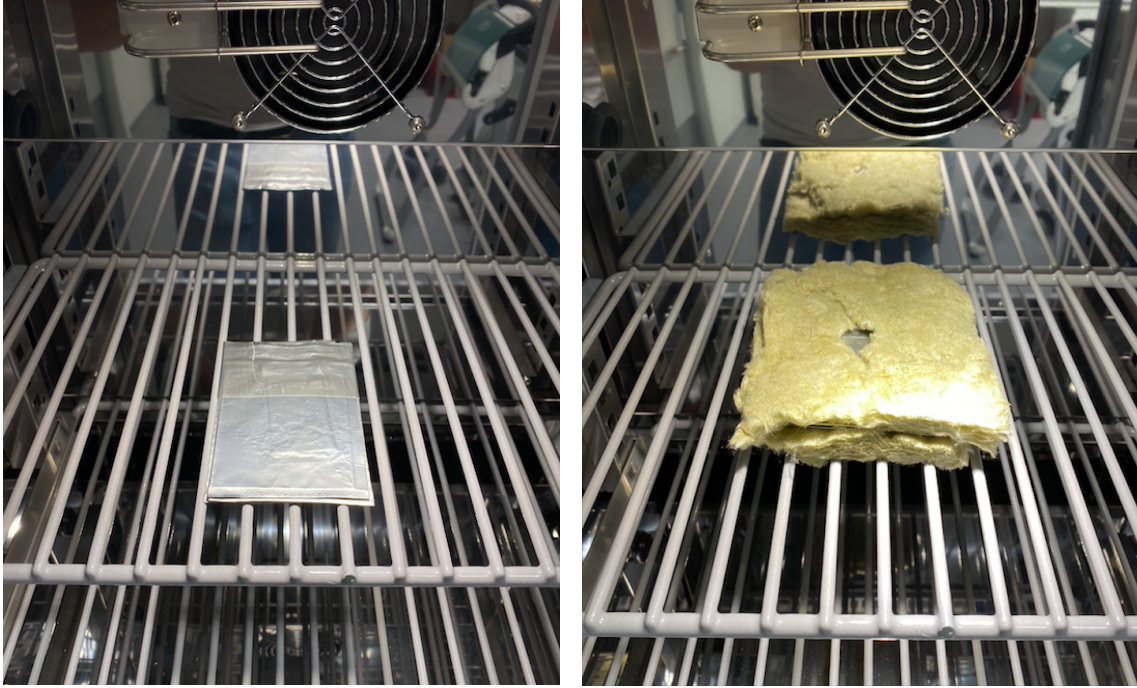
(a) The semi-solid state stack in the thermal chamber.
