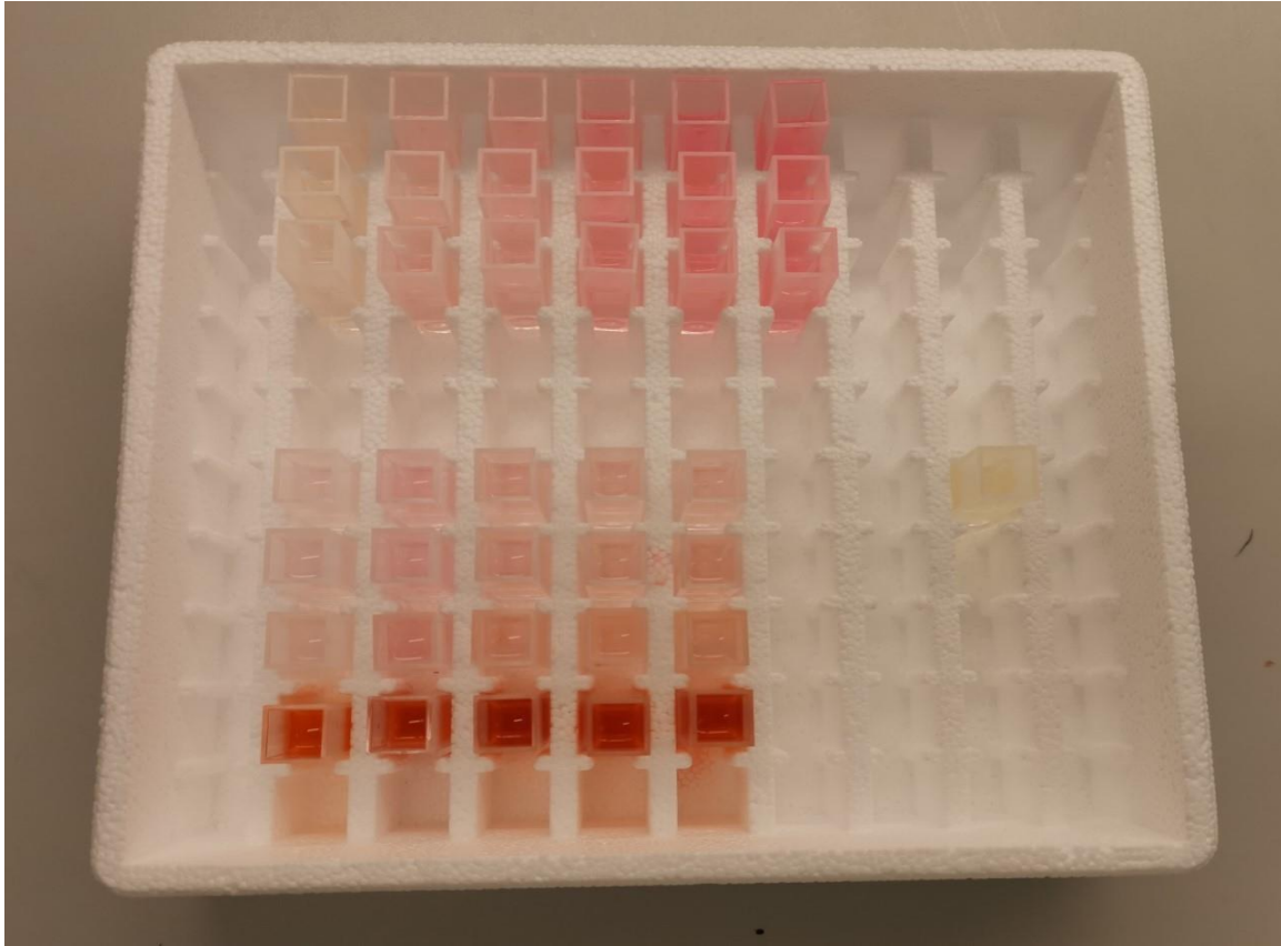
Figure 13. Cuvettes containing TBARS samples ready for spectrophotometric reading. The TEP standard graph (1, 3, 5, 10, 15, and 20 nmol/MA) can be seen in triplicates at the top. The blank sample is located to the right. The bottom row shows the oxidized oil on sampling days 0, 7, 14, 21, and 28, respectively. The top row in the same bulk shows the same samples diluted 1:100, which were analyzed in the spectrophotometer.
