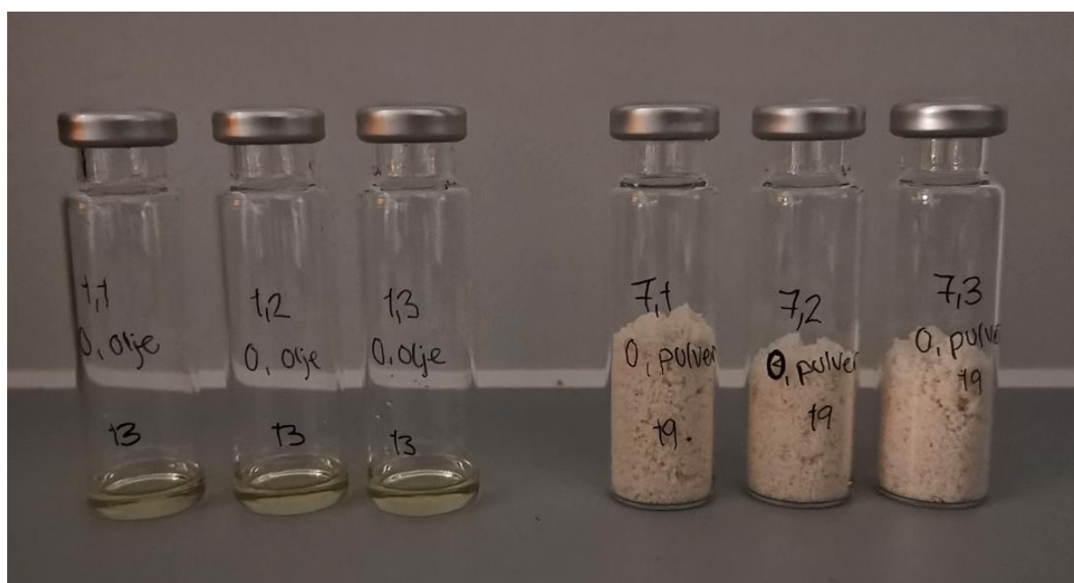
Figure 15. Illustration of GC-MS vials containing 1 mL of oil (left), and vials containing 1 g powder (right).
