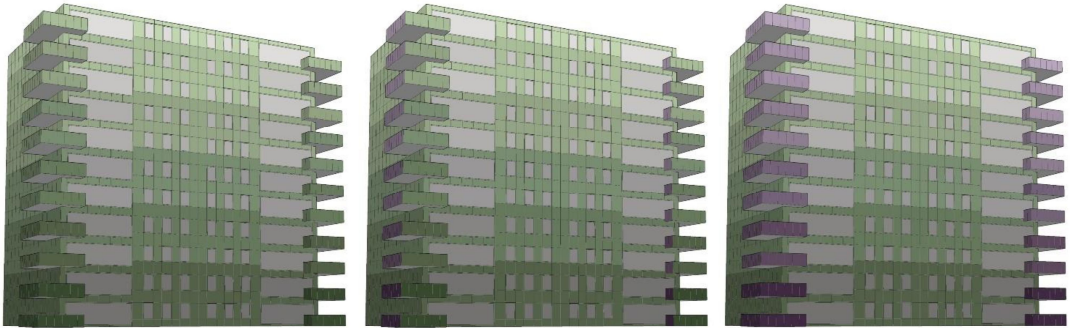
Figure 40. FIPV design for high-rise with side small balconies, in main greenish hue G30Y and the corresponding complementary hue
