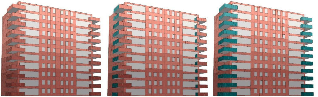
Figure 39. FIPV design for high-rise with side large balconies, in main reddish hue Y80R and the corresponding complementary hue
