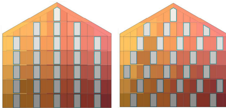
Fig. 23. Colour harmony design proposals (hue Y20R to Y90R, B and B40G with chromaticness = 50).
