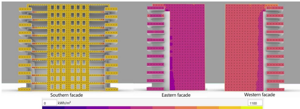
Figure 29. Solar radiation mappings for high-rises with side large balconies.
