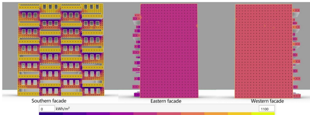
Figure 27. Solar radiation mappings for high-rise buildings with staggered large balconies.
