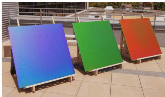
Figure 2.24: Demonstrator coloured modules by Fraunhofer Institute for Solar Energy Systems ISE. From Bläsi et al. (2021) 20
