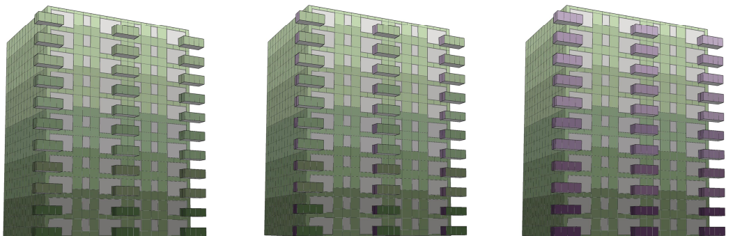
Figure 37. FIPV design for high-rise with side small balconies, in main greenish hue G30Y and the corresponding complementary hue
