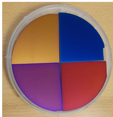
Figure 2.25: Coloured prototypes with thin-films applied on top of flat Si wafer solar cells, from Ørnulf Nordseth. 21
