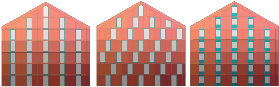
Fig. 22. Split complementary colour harmony design proposals (hue Y70R, Y80R, Y90R and B40G with chromaticness = 50).
