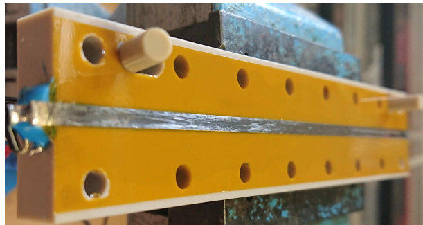
Figure 3.10: Bottom Plate 2 with Kapton tape. The two pegs at either end are for alignment of top and bottom plates. Image is rotated 90° clockwise from photograph.
