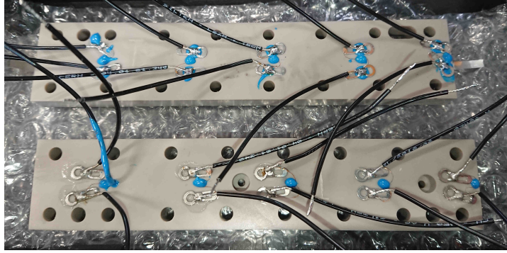
Figure 3.4: Top Plate and Bottom Plate 1 after installation of heater strip, Eccobond® filling of sensor lead holes, and attachment of sensor leads and sensor lead extensions to soldering pads.
