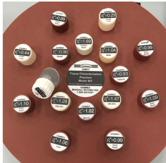
Figure 3.1: Gammex 467 Tissue Characterization Phantom.
