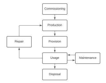
Figure 3.2: The life of an asset, adapted from DIN SPEC 9134:2016 [2016]
