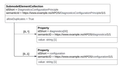
Figure 5.5: Contents of the nested SMC with idShort "DiagnosticsConfigurationPrinciple" of the SMC with idShort "EquipmentAttributes" in figure 5.2.
