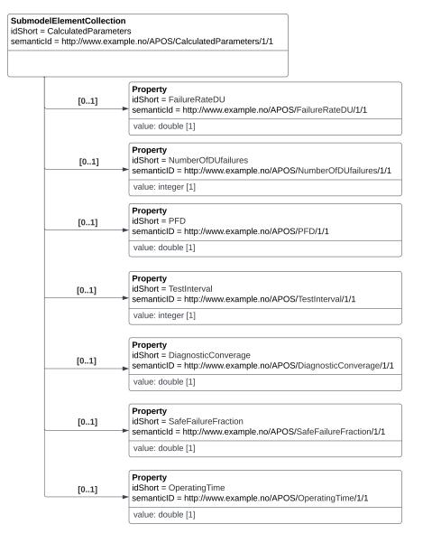
Figure 5.10: Contents of the submodelElementCollection with idShort "CalculatedParameters" of the submodel template with idShort "FailureReport" in figure 5.8.
