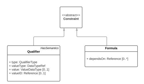
Figure 4.3: Inheritance from Constraint, adapted from Plattform Industrie 4.0 and ZVEI [2020a].
