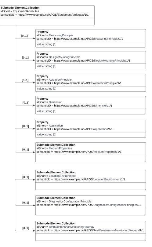
Figure 5.2: Contents of the SMC with idShort "EquipmentAttributes" in the submodel template for equipment group shown in figure 5.1.
