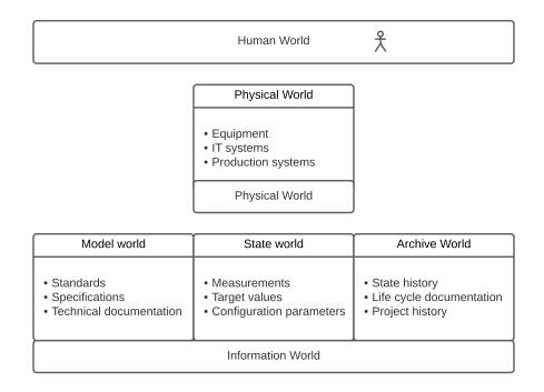
Figure 3.1: The object worlds of I4.0, adapted from DIN SPEC 9134:2016 [2016]
