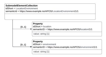
Figure 5.4: Contents of the nested SMC with idShort "LocationEnvironment" of the SMC with idShort "EquipmentAttributes" in figure 5.2.
