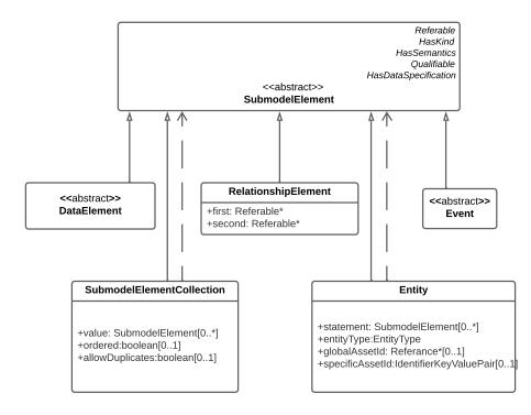
Figure 4.6: Metamodel of SubmodelElement, adapted from Plattform Industrie 4.0 and ZVEI [2020a].
