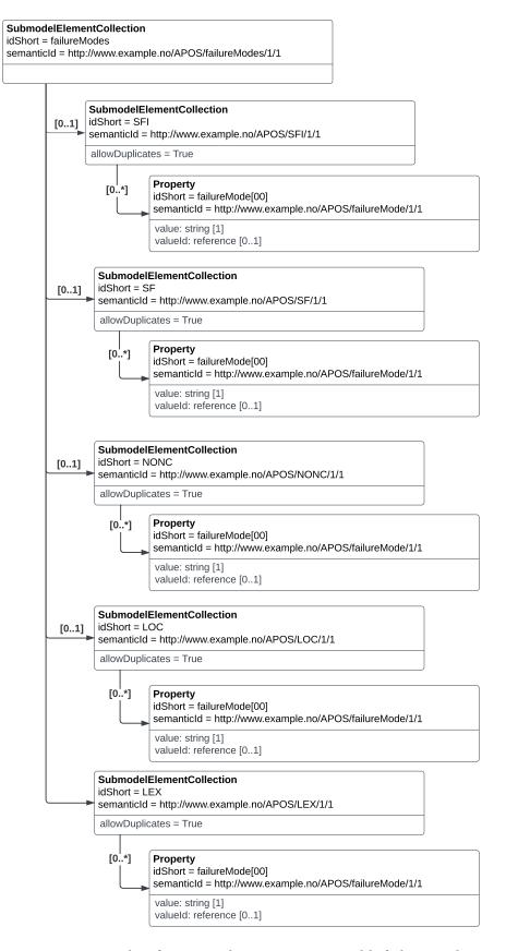
Figure 5.7: A template for a SMC that represents possible failure modes
