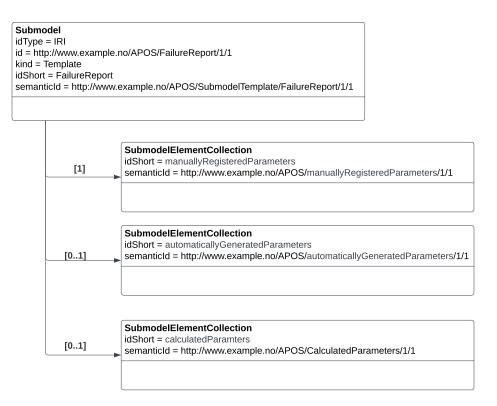
Figure 5.8: Submodel template for failure parameters
