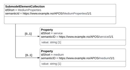
Figure 5.3: Contents of the nested SMC with idShort "MediumProperties" of the SMC with idShort "EquipmentAttributes" in figure 5.2.
