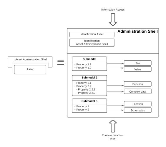
Figure 3.4: Basic structure of an AAS, adapted from Ye and Hong [2019]
