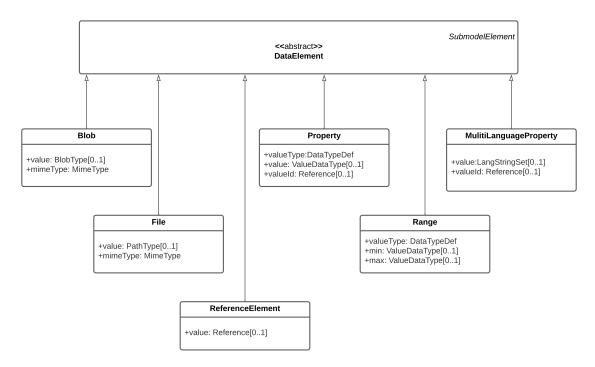
Figure 4.8: Metamodel of DataElement, adapted from Plattform Industrie 4.0 and ZVEI [2020a].
