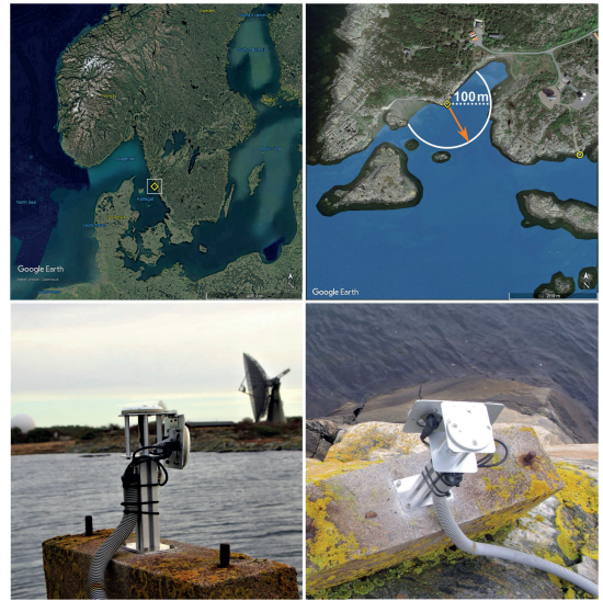
Fig. 1. (Top Left) Top view of the Onsala GNSS-R station located in southern Sweden. (Top Right) Nearby coastlines. (Bottom Left) Close eastward. (Bottom Right) Downward photographs from the antennas and the setup structure. The GNSS-R station is marked with a yellow diamond, and the yellow circle shows the location of the nearby tide gauge station. The orange arrow indicates the boresight of the reflectometry antennas.
