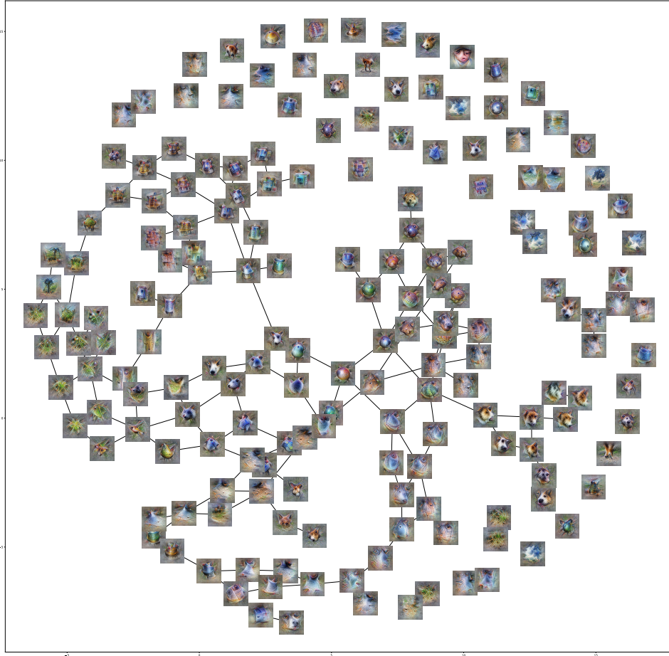
FIGURE 41. A Mapper Activation Atlas of P_{4c} . Projection on the first two principal components is used as the filter function. The cover is balanced , 6 \times 6 rectangles with 0.1 overlap. The clustering used is k -means clustering with k = 5 . The \min\_intersection is 40.
