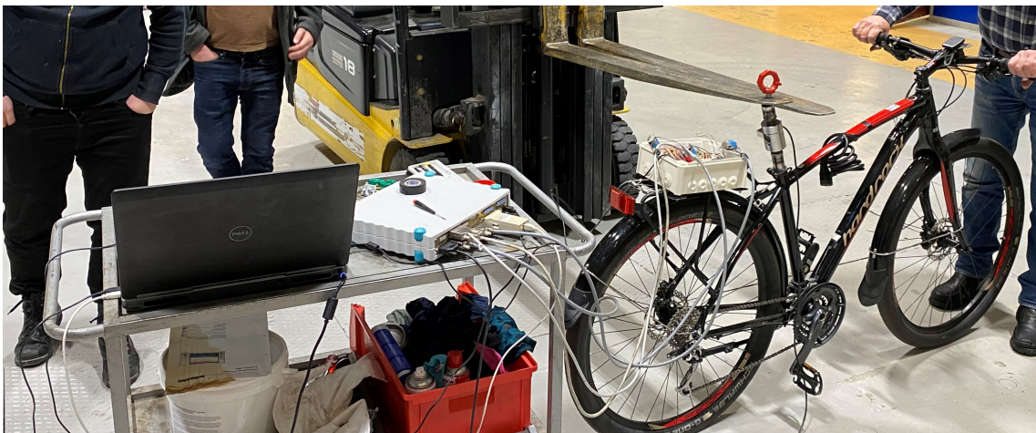
Fig. 6.2. Placing weight onto the bicycle seat using a forklift.
