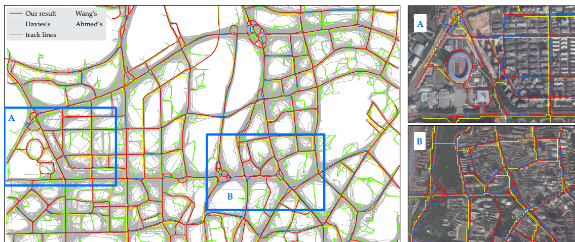
Figure 12. Overlaying the road networks extracted by our method and another three methods from [27,34,39].
