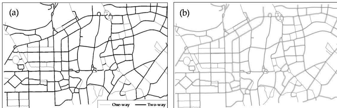
Figure 11. Driving rule identification of one-way and two-way road segments: (a) driving rules identification; (b) two-way road reconstruction.
