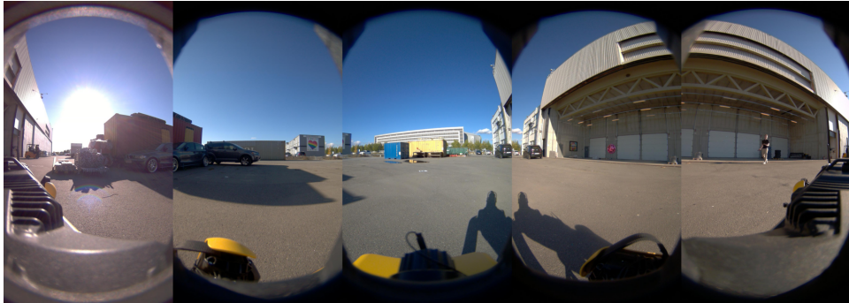
Figure 3.11: The view of the five fisheye cameras. Notice the severe radial distortion effect in the images.
