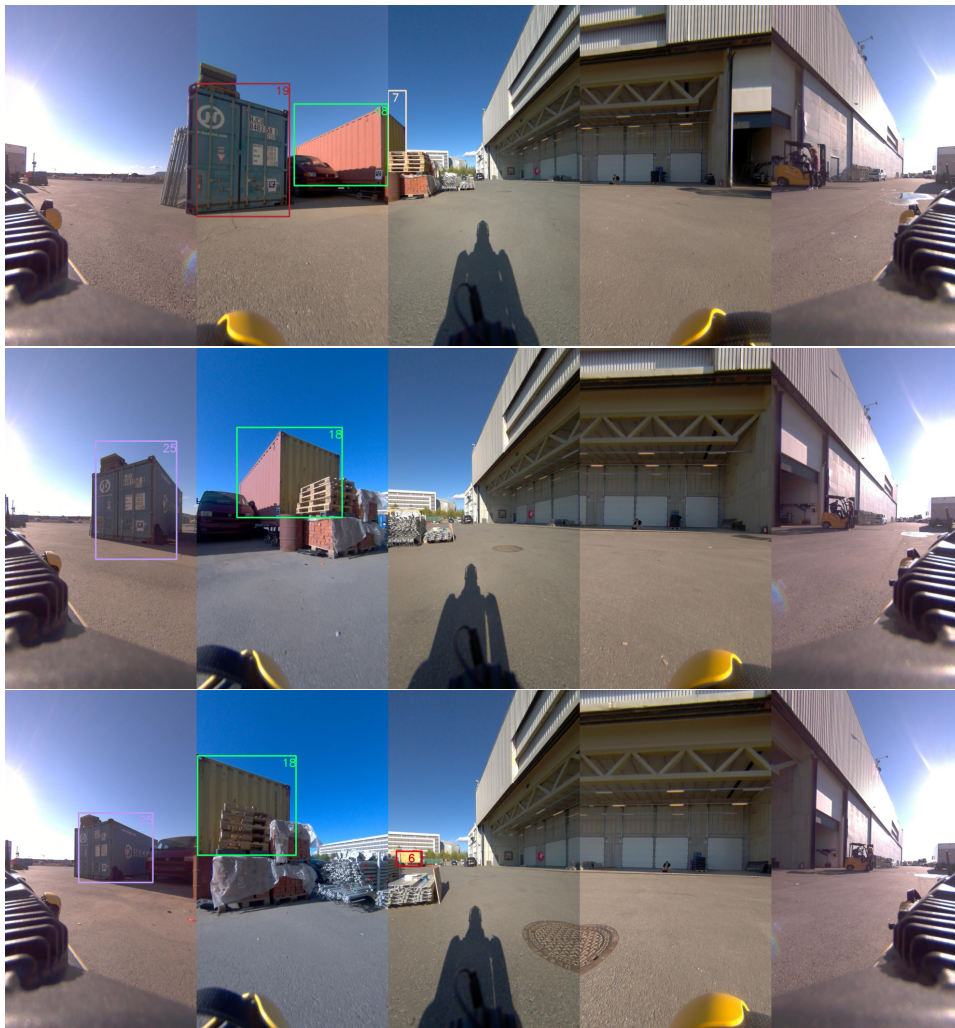
Figure 3.15: Five unique tracks for the first, fifth and tenth frame in a video sequence. Track IDs are found in the top right corner of the bounding boxes.
