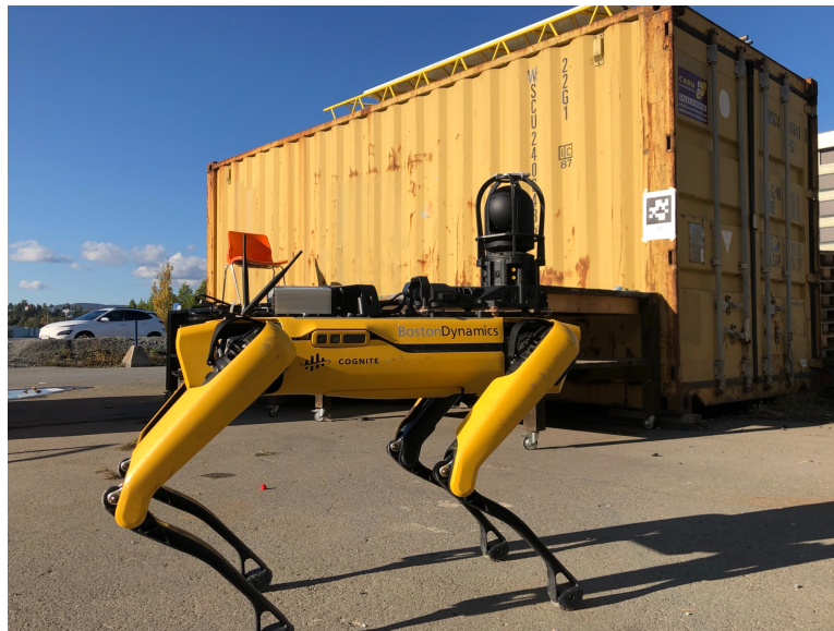
Figure 3.2: The Spot robotic platform was used in this work. The SpotCAM+ payload on the front and the SpotCORE on the robot's rear.
