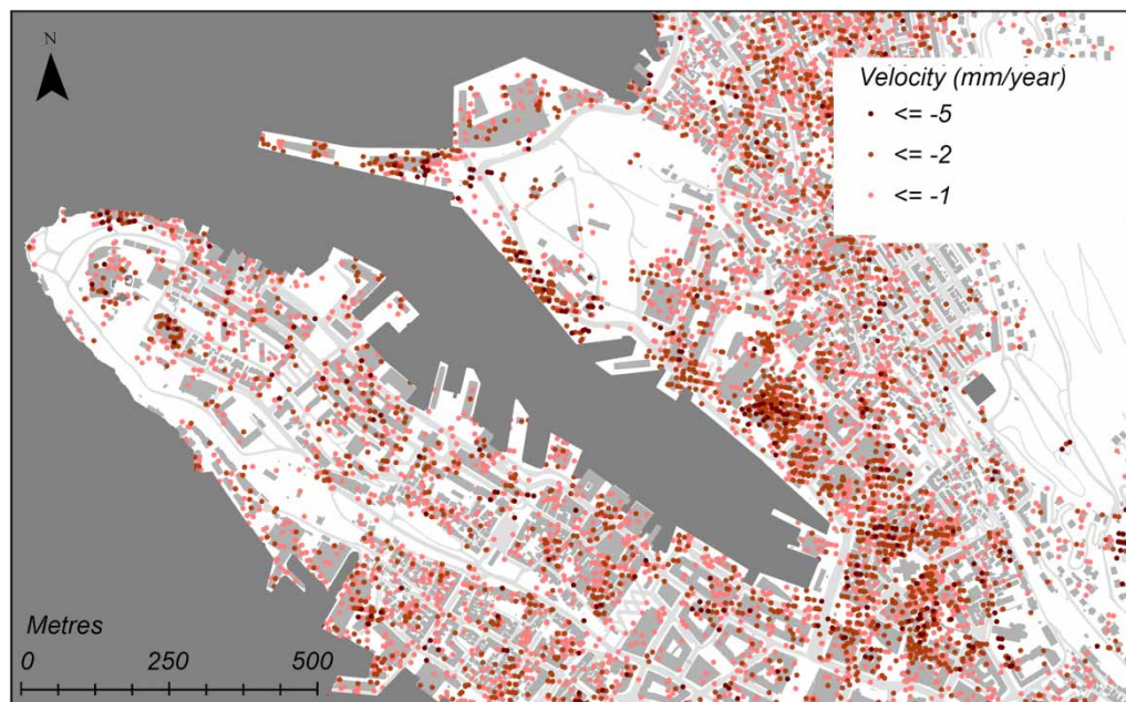
Figure 5 | PSI data from Sentinel-1 for the time period 2015–2018 collective ground movement, subsidence (vertical velocity) in mm/year. Data from the Norwegian Map Authority (2018). Please refer to the online version of this paper to see this figure in colour: http://dx.doi.org/10.2166/nh.2019.030 .
