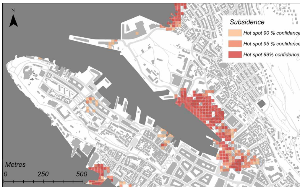
Figure 9 | 'Hot spot analysis' where clusters of subsidence are within areas of pluvial or coastal flooding. The grid cells are 20 \times 20 m. Please refer to the online version of this paper to see this figure in colour: http://dx.doi.org/10.2166/nh.2019.030 .
