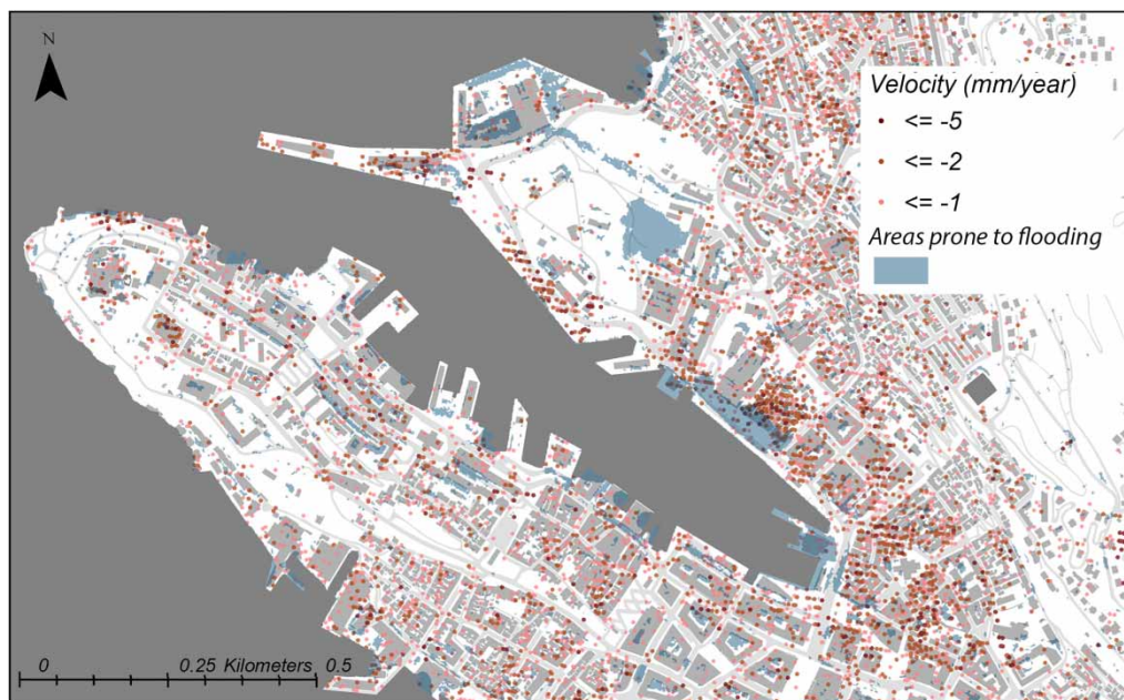
Figure 7 | The PSI data indicates that subsidence is shown in red and the flooded areas in blue. With an overlay of the two datasets, the map shows a city widely affected by subsidence as for areas prone to flooding. Please refer to the online version of this paper to see this figure in colour: http://dx.doi.org/10.2166/nh.2019.030 .
